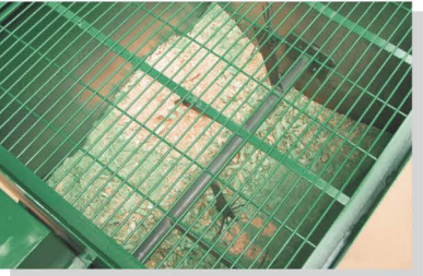
awdust bunker with sifting grate, mixer and sneck for sawdust dosing in the drying-burning chamber
